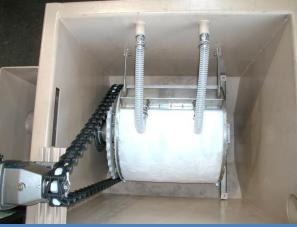
Wastewater Technologies continues to expand its liquid/solid separation capabilities by adding a user-friendly, small footprint, low backwash, high performance tertiary filter for both small and large flow applications. The **BioDRUM™** Cloth Media Filter removes suspended solids as small as 10 microns and can be configured for flows as low as 4,000 GPD up to 165,000 GPD.
